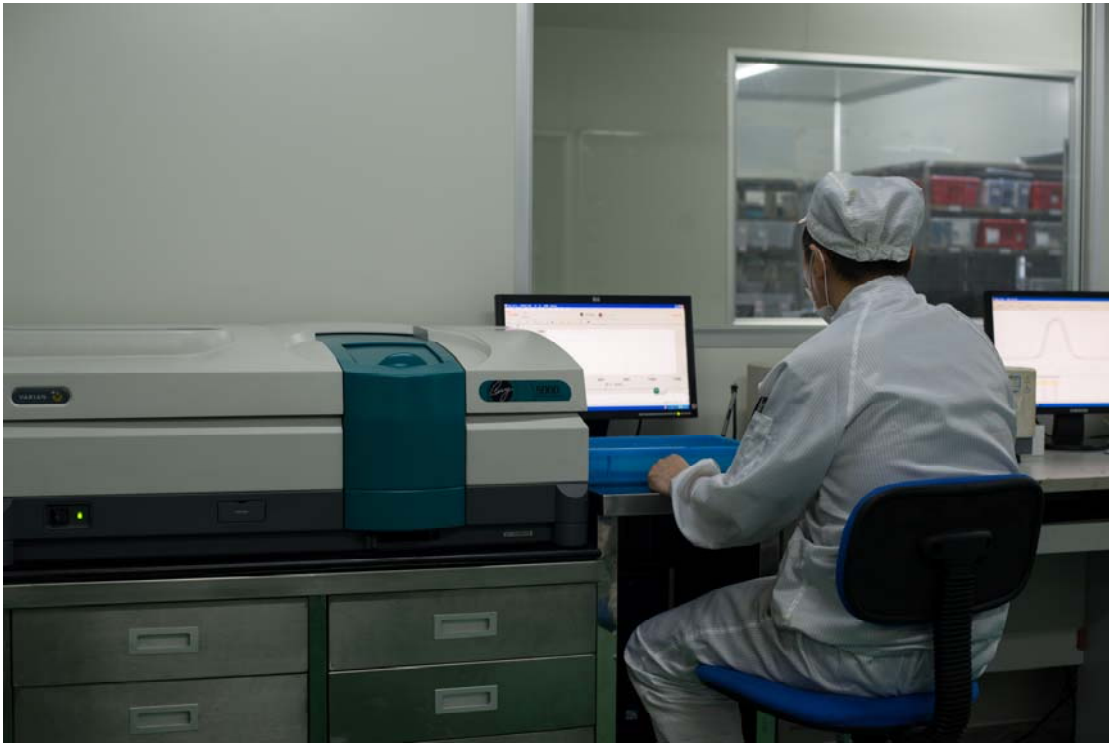
Cary 5000 Photospectrometer for measuring transmission, OD6 of optical depth can be recognized
