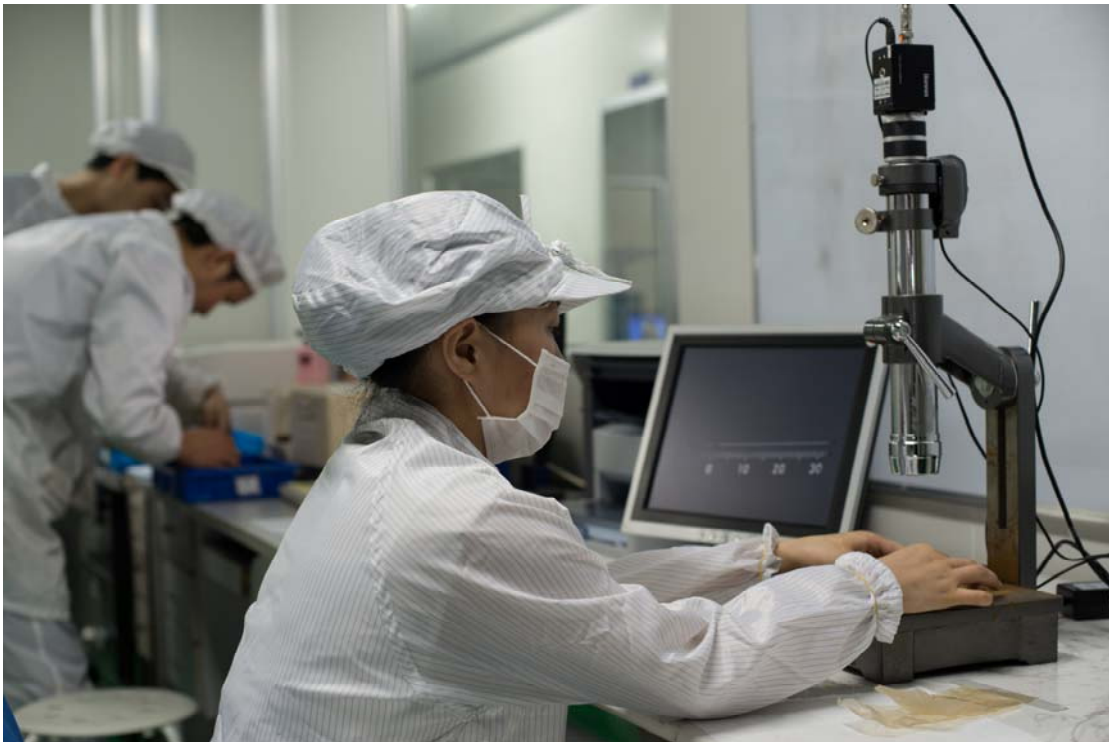
Collimator for testing cubes beam deviation
